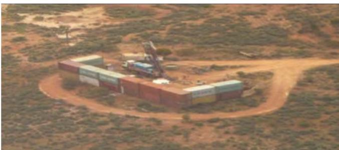
Figure 1: Sea containers create a noise barrier around a drill rig
